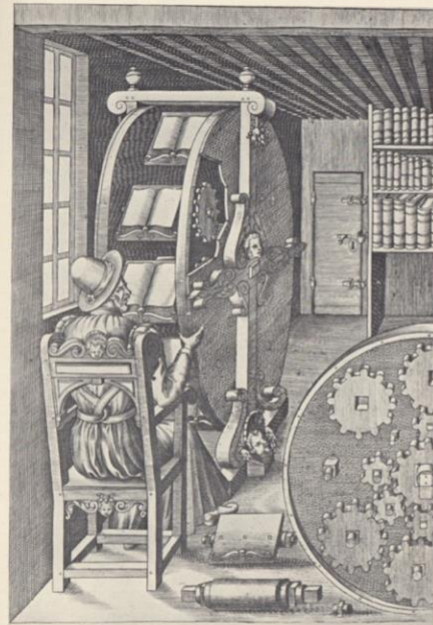
Fig. 68c. The source of the illustration used by Johann Schreck & Wang Ching, the revolving bookcase depicted in Ramelli's engineering treatise of +1588. A simple arrangement of gearing keeps the successive book-rests at the same angle as they are rotated. From this it can be seen that the Chinese draftsman of Fig. 679 drew the gear-wheel system erroneously.
